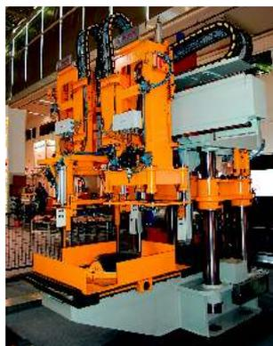
»1 IP131 hydraulic press for accessory roofing tiles and special
