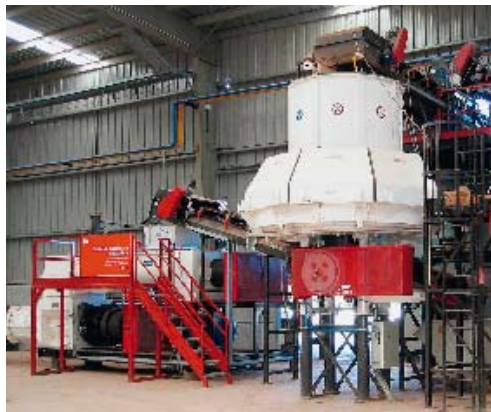
» Händle shaping plant for roofing tiles with circular screen feeder type BRSH 19b, extruder E 65a/ 60 and de-airing double-shaft mixer type MDVG 1025f
